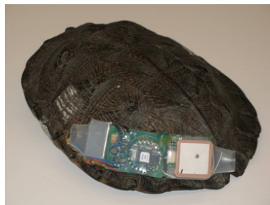
Figure 6: The energy measurement and charging board with a Mica2Dot, GPS receiver, and battery.
